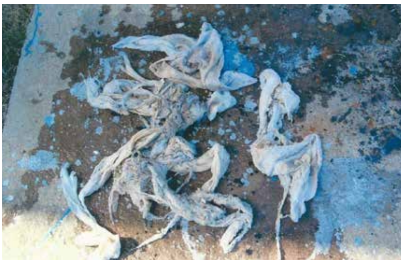
"Flushable" wipes that were causing issues and were pulled from a wastewater collection system in South Dakota.
